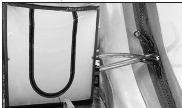
Figure 12 – Sealing test in NHC.
