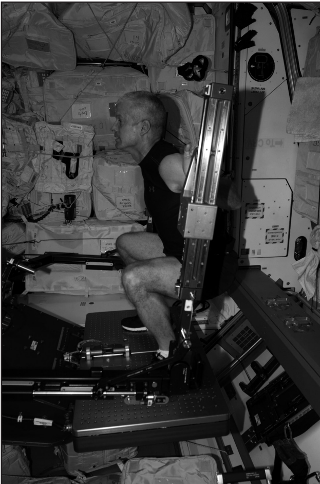
Figure 4 - Advanced Resistive Exercise Device (ARED).
