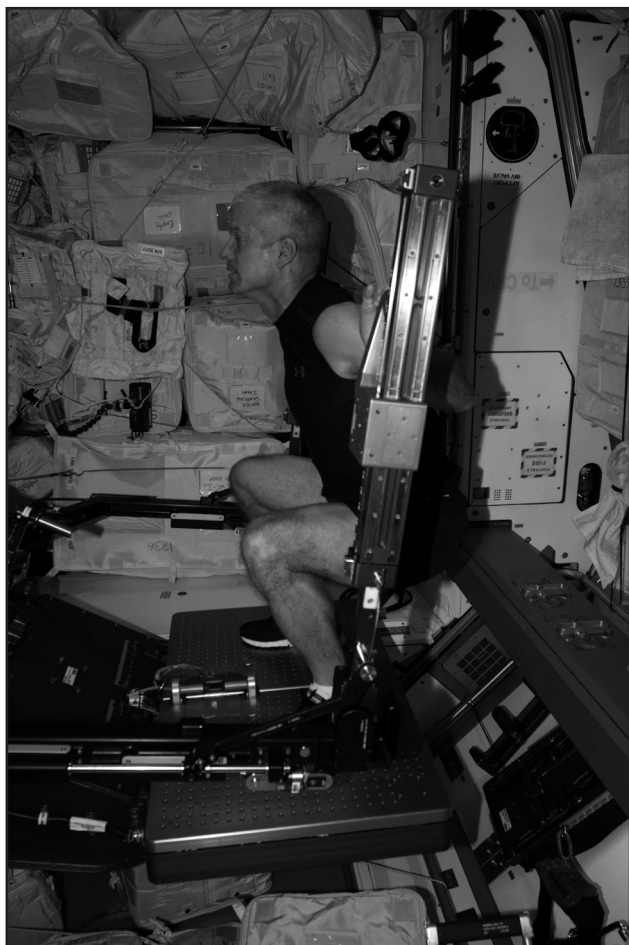
Figura 4 - Advanced Resistive Exercise Device (ARED) .
