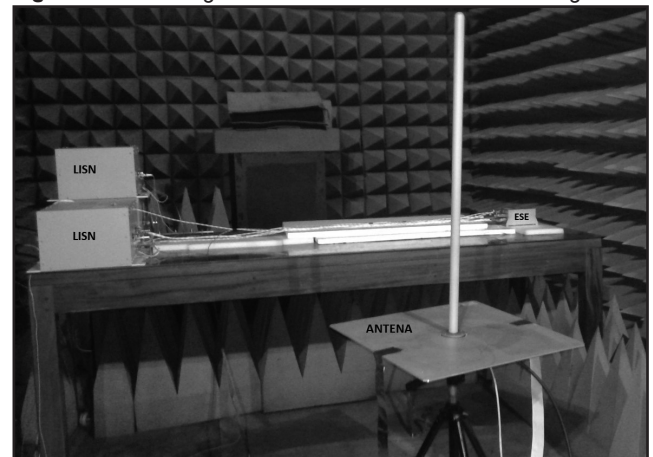
Figure 9 - Positioning of the ROD antenna for RE-102 testing.
