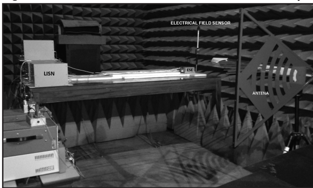
Figure 14 - BICONILOG antenna for RS-103 test run in laboratory.
